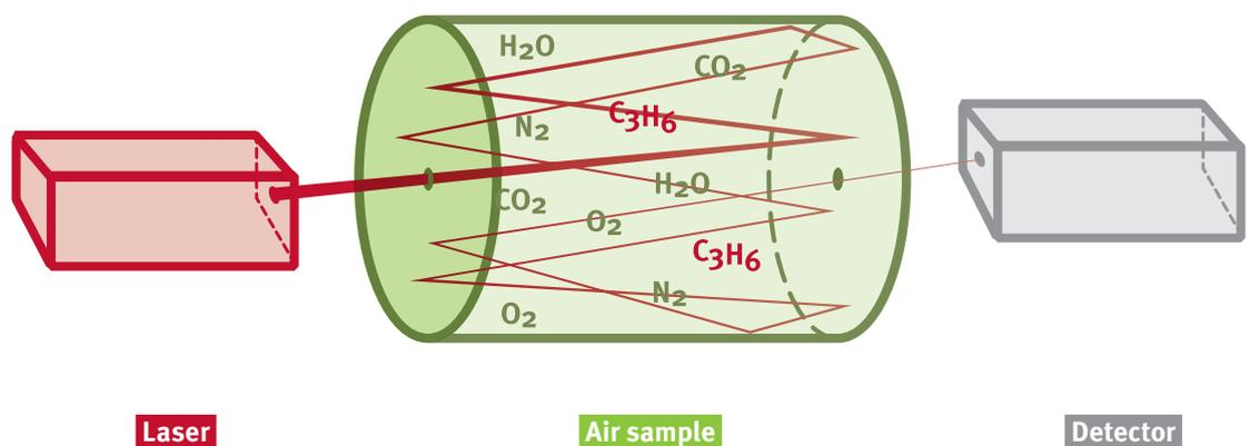
cules – in this case acetone molecules. Lower light intensity on the detector thus indicates a higher acetone concentration in the investigated air sample. This method has the advantage of dispensing with the need for the time-consuming preparation of samples in the laboratory and can produce the measurements within minutes.
